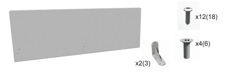
Start by assemble the brackets to the screen. Use the M8 screws in the burnt holes, 2xM8 / bracket. Don't tighten the screws to hard. This will damage the chipboard and the screen will not be fixed proper to the desk.
