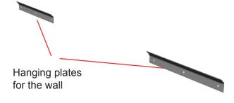
Screw the corresponding hanging plates on to the wall. Use proper screws for the wall material.
