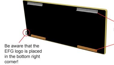
Screw the hanging plates and the distancers on the backside of the screen with wooden screws. Use the guideline holes.
