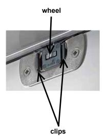
The Doors are hooked in by clip-in installation. The Doors can be removed by pressing the two flanges on the fitting toward each other and pull out.
