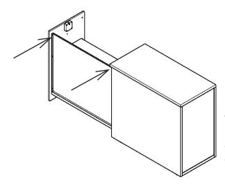
Pull out the inside part fully. Remove the two upper most screws that fixate the metal side, one against the back and one against the front. Use a 2,5 mm allen key and loosen the screws.
