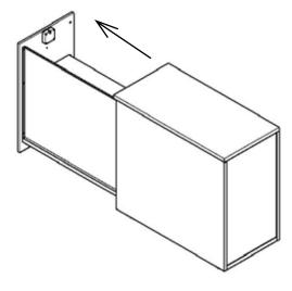
Pull out the inside part fully. To remove the metal side, on the inside unit, use a 2,5 mm allen key and loosen all screws that holds the metal side. 6 pcs for the low tower and 8 for the high.
